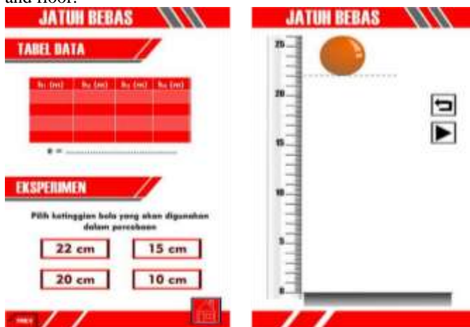
Figure 4 Screenshot of the Simulation about Collision between a Ball and the Floor. The Ball is Released from a Certain Height without Any Initial Speed. Students are Asked to Determine the Restitution Coefficient
